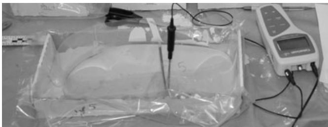
FIG. 2—The experiments array—the thermometer is placed in one dental stone cast.
